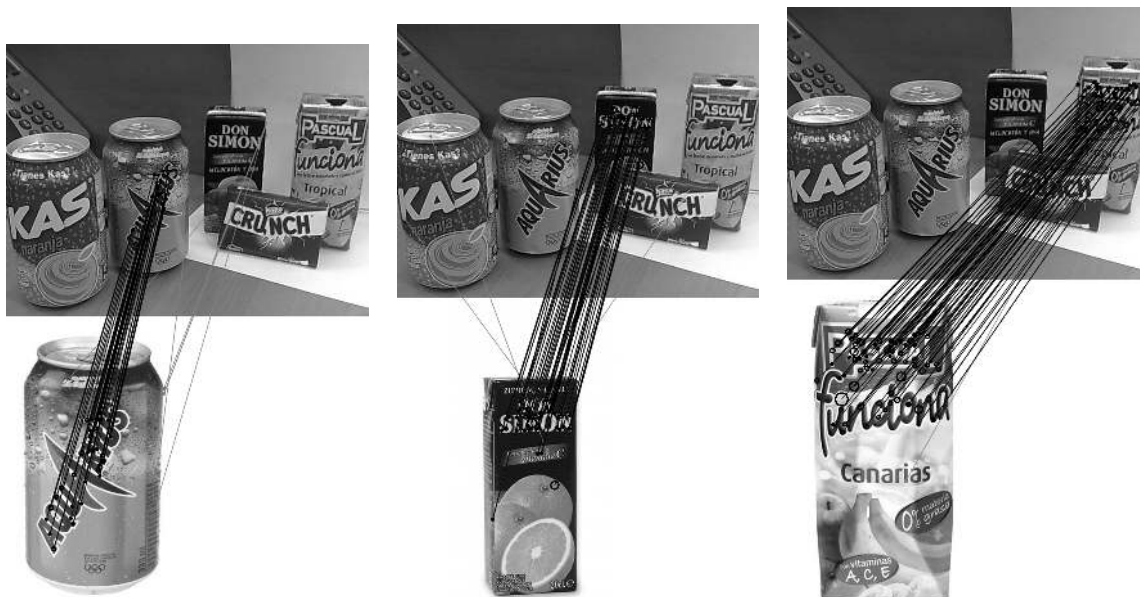
FIGURE B.5: Example of the use cases where many objects are present in the scene (see section 6.6). The inliers are coloured in black, the outliers – in grey.
